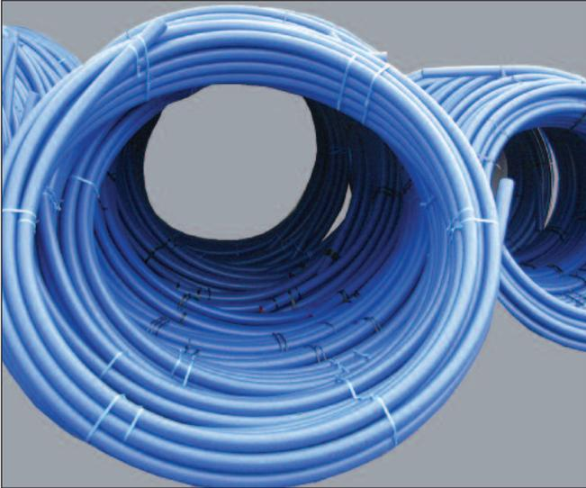
Blue and black medium density (PE80) polyethylene service pipes suitable for potable water and industrial uses. Kitemark certified to BS EN 12201.
